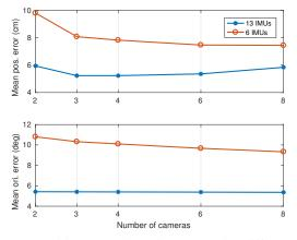
Figure 3: Position and orientation error with different sensor configurations, 13 or 6 IMUs and 2-8 cameras. Sequence: S2 - FS1, SS 1/1.
