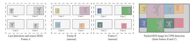
Figure 2: Visualization of the ROI packing process for efficient multi-camera/frame CPM detection.
