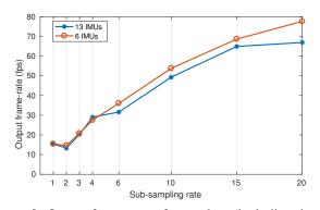
Figure 8: Output frame-rate of our solver (including detections) as a function of sub-sampling level. Sequence: S2-FS1, 4 cameras,  $N_o = 2$ .
