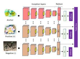
Figure 1. The triplet convnet for learning the style model comprises three fully shared (siamese) branches formed from GoogleNet with a bottleneck layer appended to pool5. Training proceeds via classification loss, followed by triplet loss guided by hard negatives exhibiting shared semantics and differing style.
